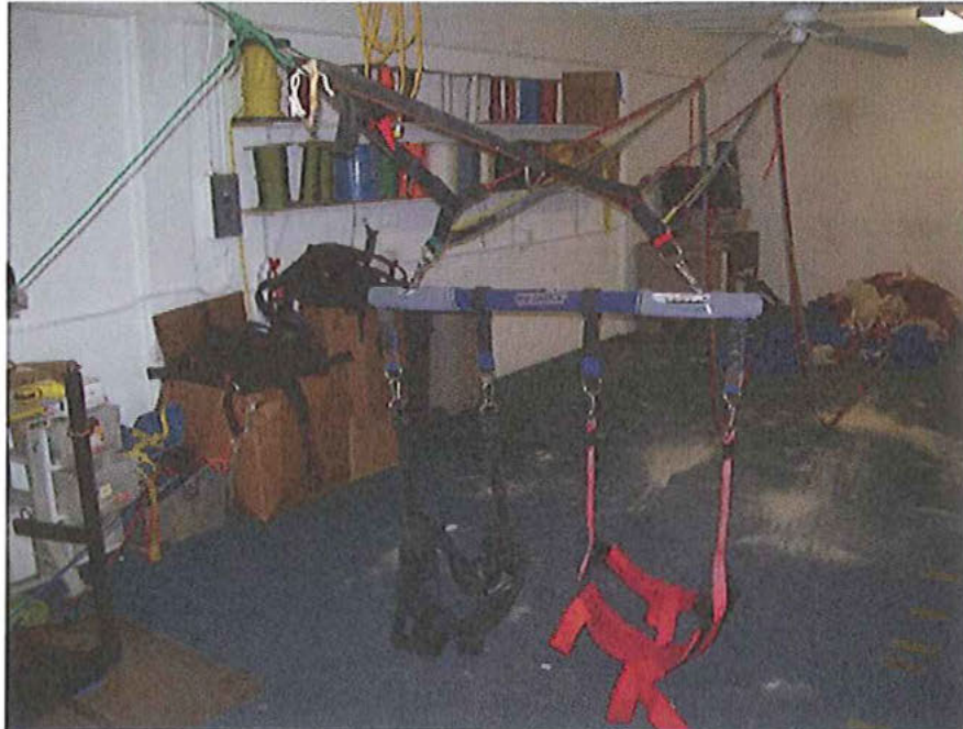
Figure 05. Representative picture of parasailing components as they would be with passengers in flight. (Not actual equipment used on M/V TURTLE)
